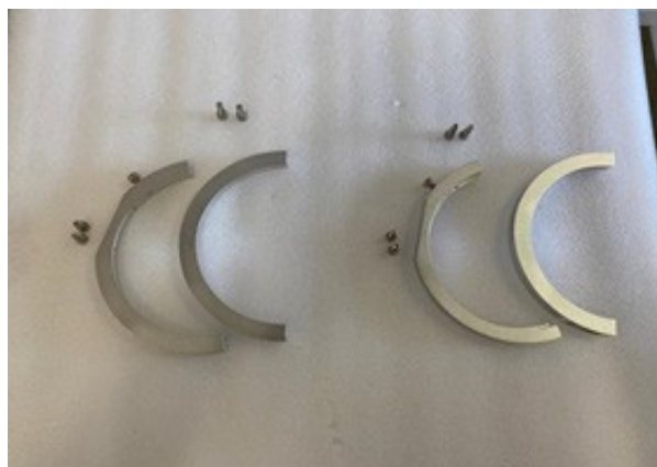
Figure 18.3.b: Trunnion Rings Unscrewed
