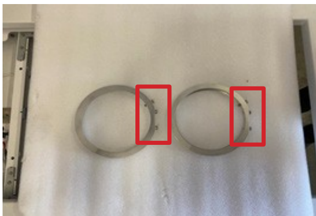
Figure 18.3.a: Trunnion Ring Screws
