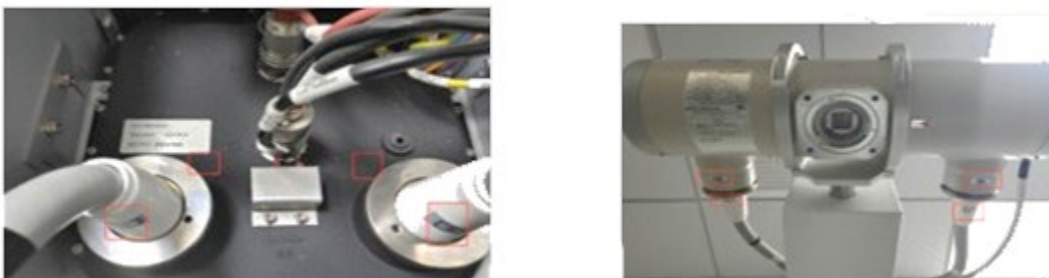
Figure 22.1: Showing connection between SMART HF generator and X-ray tube using high voltage cables and rotating anode
