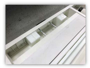
2. Remote outside of double sided tape on base inserts and inset into sides of panel enclosure:
