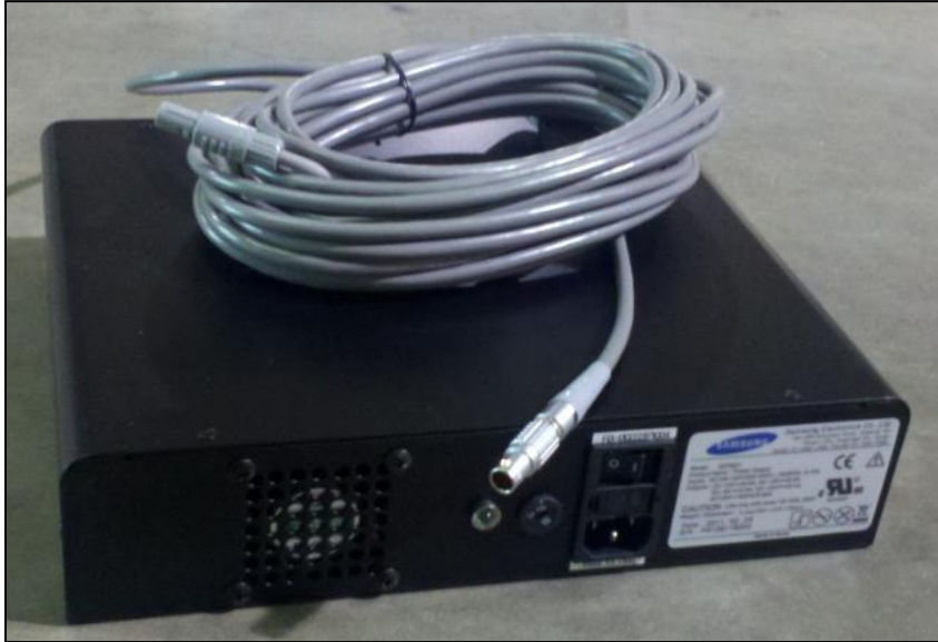
Figure 1.3 - Panel Power Supply plus Power Supply Cables
