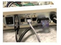
3. Connect the Exposure Switch from the Base cable assembly to the Exposure connector.
