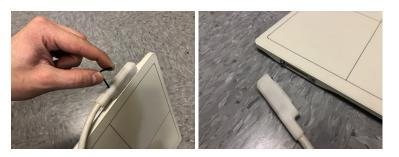
3. Route tether cable through designated grommet(s) to go inside of the base for cable management.
