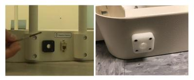
2. Disconnect the tether cable from the DR panel, 2 1.5mm (or 5/64) allen screws
