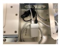
6. Connect the other end of the 3' Ethernet Cable(s) to the back of the base.
