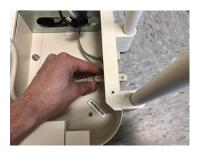
4. Place A/C Adapter(s) for DR panel(s) inside base and connect adapter power, as well as panel power connector to A/C adapter (left – Single panel, right – Dual panel).
