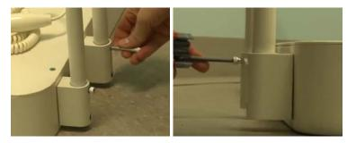
2. Secure the Patient Back Handrail (C) to the back side of the Podiatry Base (B) from the outside using 4 ea. 1/4-20 x 2" SHCS. Tighten securely.
