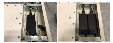
5. Connect both the 3' Ethernet (RJ-45) data connection(s) and Power connection(s) to the splitter.
