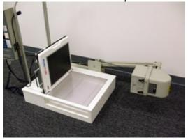
\*Position the Tube Head (attached to swinging arm) for a lateral shot, except make the center of the tube head level with the center of the panel.
