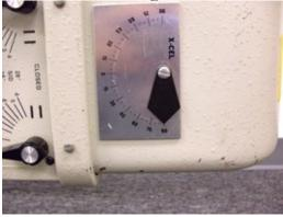
\*You can check to be sure it is centered by turning on the light field, and expanding the columnators, but only to the amount of about 10x12"
