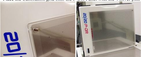
\*NOTE: if the grid will not go on because it is hitting at the bottom at the base, be sure what your using to raise the panel up is tall enough
